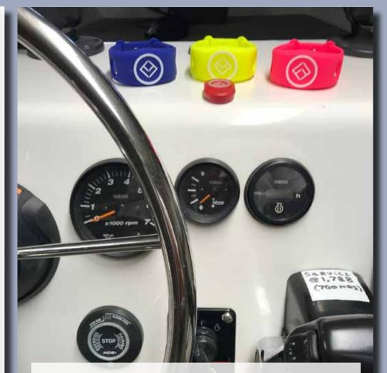
The SKIFF program's boat has been equipped with the MOB+ Wireless Man Overboard System. The hub (round gauge marked "STOP" on lower left) mounted in the dash communicates with small fobs (small red device in front of yellow wristband) which may be placed inside wristbands (shown in blue, yellow, and pink). Fobs may either stop the boat or sound an alarm when they stray more than 50 feet from the hub and/or submerge more than 4 inches.
